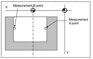
To set the workpiece coordinate offset, the position X (position Y, position Z) of the measurement A point is measured, and the measured value is set in the measurement A point. In the same manner as the measurement A point, the measurement B point is measured and set.
