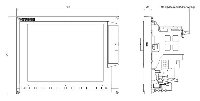
(Note) The space of 30mm or more should be provided above the display unit for maintenance.
