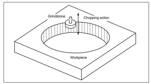
The chopping operation is initiated by setting the upper dead point position, lower dead point position and number of cycles (number of up/down movements per minute) and pressing the chopping start switch.
