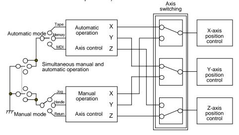
The feed rates for the axes subject to automatic commands and the feed rates for axes subject to manual command are set separately. The acceleration/deceleration modes (rapid traverse, cutting feed) are also set separately. Rapid traverse override, cutting feed override and second cutting feed override are valid both for axes subject to automatic commands and manual commands.
