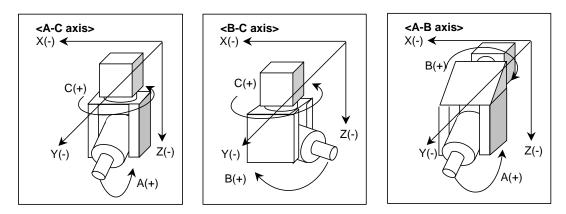
This is also effective for a machine configuration having the tool tilt 1 axis and table tilt 1 axis.
