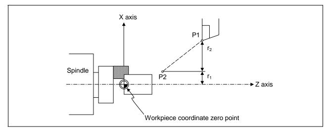
When the tool is to be moved from point P1 to point P2
