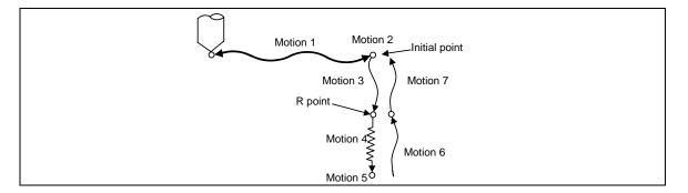
The drilling cycle motions generally are classified into the following seven.
