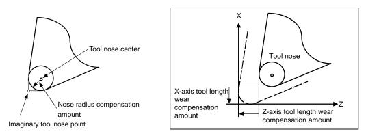
The X-axis tool length compensation amount, Z-axis tool length compensation amount and nose radius compensation amount are set as plus amounts.
