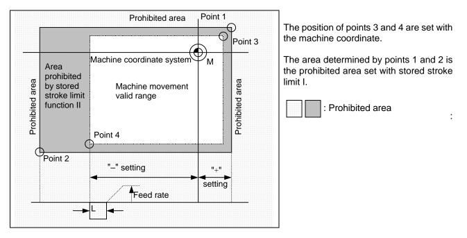
All axes will decelerate and stop if an alarm occurs even for a single axis during automatic operation. Only the axis for which the alarm occurs will decelerate and stop during manual operation. The stop position must be before the prohibited area.
