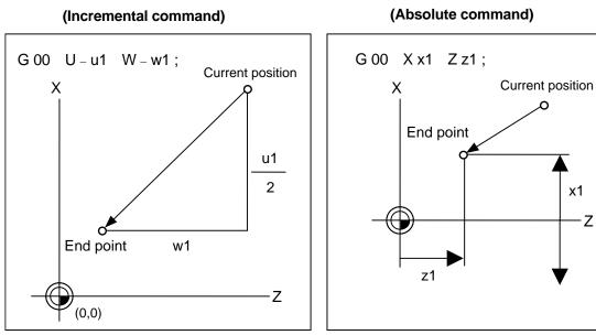
The above drawing shows the case for the diameter command.
