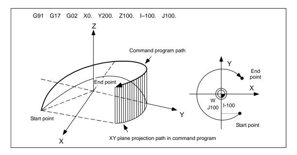
(Note 1) Helical shapes are machined by assigning linear commands for one axis which is not a circular interpolation axis using an orthogonal coordinate system. It is also possible to assign these commands to two or more axes which are not circular interpolation axes.
