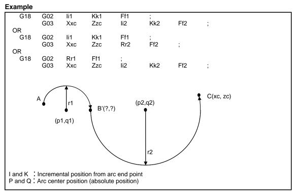
I and K are the arc center position (incremental position); distances from the start point in the first block or distances from the end point in the second block. P and Q (X, Z arc center position (absolute position)) can be commanded instead of I and K commands.
