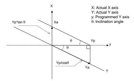
Yp, the Y-axis position on the programmed coordinates (on the orthogonal coordinates), is the position of Xa and Ya which are produced by synthesis of X axis and Y axis.
