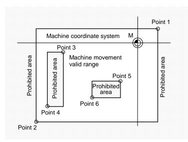
The area determined by points 1 and 2 is the prohibited area set with stored stroke limit I.
