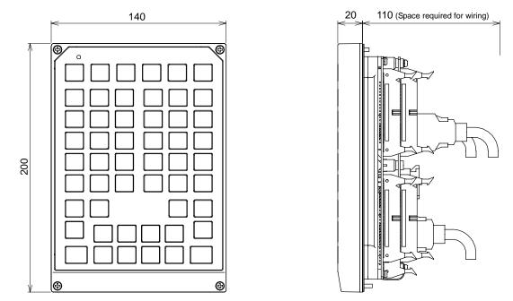
(Note) The above side view shows the state with the Operation panel I/O unit FCU7-DX720/DX721 mounted.
