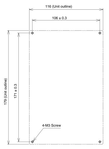
(Remarks) When using FCU7-KB024/FCU7-KB026/FCU7-KB044, the Operation panel I/O unit can be mounted on the back of the keyboard.
