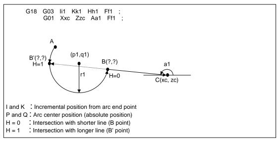
The p1 and q1 can be commanded instead of li1 and Kk1. The arc - linear contact is automatically calculated by designating R instead of I and K (P, Q).
