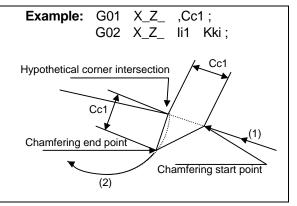
(b) Corner chamfering II (Circular - linear)
