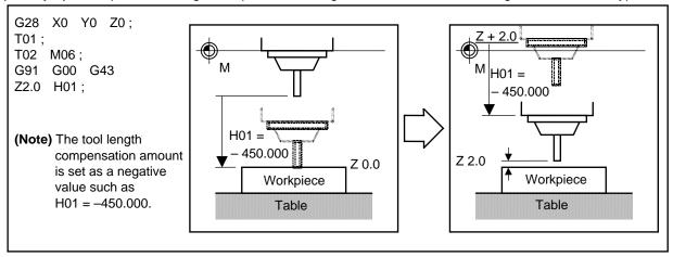
(Example) Example of tool length compensation using a combination with tool length measurement type I
