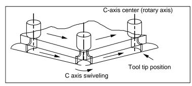
During arc interpolation, the C axis turning is controlled in synchronization with the operation of arc interpolation.
