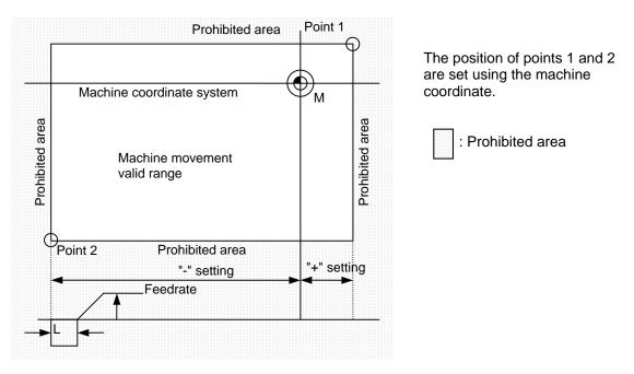
All axes will decelerate and stop if an alarm occurs even for a single axis during automatic operation. Only the axis for which the alarm occurs will decelerate and stop during manual operation. The stop position must be before the prohibited area.
