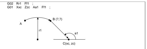
The arc - linear intersection is automatically calculated by designating R instead of P and Q (I, K).
