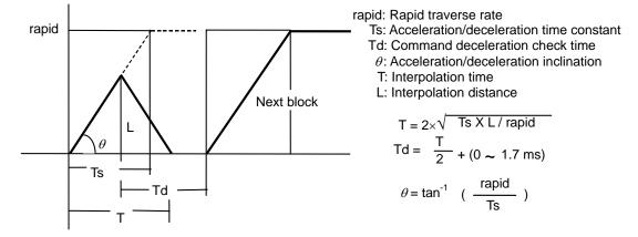
The time required to perform a command deceleration check during rapid traverse constant inclination acceleration/deceleration is the longest value among the rapid traverse deceleration check times determined for each axis by the rapid traverse rate of commands executed simultaneously, the rapid traverse acceleration/deceleration time constant, and the interpolation distance, respectively.
