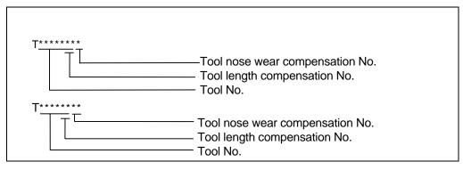
The tool compensation for the lathe is valid only for the X and Z axes. If an additional axis (Y axis) is added, the tool compensation will be validated for the additional axis.
