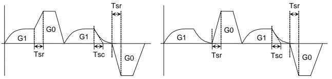
If the G0 command direction is the same as that for G1, whether G1 is to be decelerated is selected using a parameter.
