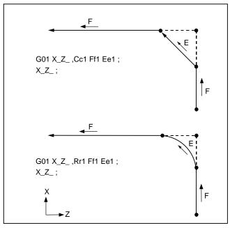
An E address is a modal and remains effective for feeding in next corner chamfering or corner R. An E address has two separate modals: synchronous and asynchronous feed rate modals. The effective feed rate is determined by synchronous (G95) or asynchronous (G94) mode.
