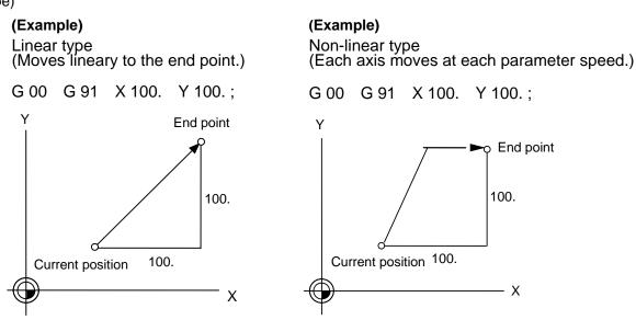
(4) The tool is always accelerated at the start of the program command block and decelerated at the end of the block.
