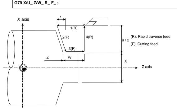
r: Taper part depth (radius designation, incremental position, sign is required)
