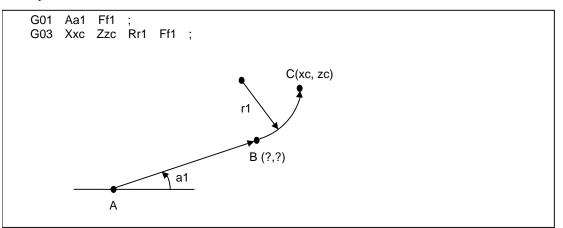
The linear - arc intersection is automatically calculated by designating R instead of P and Q (I, K).
