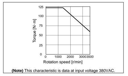
In the rapid traverse constant inclination acceleration/deceleration method, the acceleration has been treated constantly because this torque characteristic is not considered. So, It is necessary to use a minimum acceleration within the used speed range. Therefore, the margin of acceleration must be had in a low-speed range. Or if the acceleration is used to its maximum, the upper limit of the rotation speed must be slowed.
