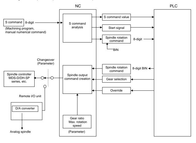
(1) The override can be designated as 50% to 120% in 10% increments or 0% to 200% in 1% increments (with built-in PLC specifications).
