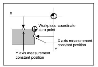
To set the workpiece coordinate offset, the X axis is measured and the X axis' offset coordinate is set. Then, the Y axis' offset is measured and set. Finally, the Z axis' offset is measured and set.
