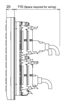
(Note) The above side view shows the state with the Operation panel I/O unit FCU7-DX720/DX721 mounted.
