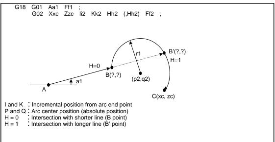
The p2 and q2 can be commanded instead of li2 and Kk2. The linear - arc contact is automatically calculated by designating R instead of I and K (P, Q).
