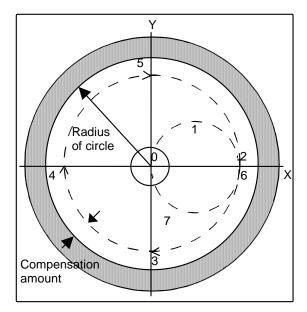
When the G12 command is used (path of tool center)  $0 \rightarrow 1 \rightarrow 2 \rightarrow 3 \rightarrow 4 \rightarrow 5 \rightarrow 6 \rightarrow 7 \rightarrow 0$ When the G13 command is used (path of tool center)  $0 \rightarrow 7 \rightarrow 6 \rightarrow 5 \rightarrow 4 \rightarrow 3 \rightarrow 2 \rightarrow 1 \rightarrow 0$
