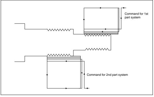
(2) 2-part System Synchronous Thread Cutting Cycle II (G76.2)
