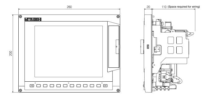
(Note) The space of 40mm or more should be provided above the display unit for maintenance.
