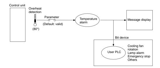
(Note 1) If the parameter is used to set the temperature rise detection function to invalid, overheating may occur, thereby disabling control and possibly resulting in the axes running out of control, which in turn may result in machine damage and/or bodily injury or destruction of the unit. It is for this reason that the detection function is normally left "valid" for operation.
