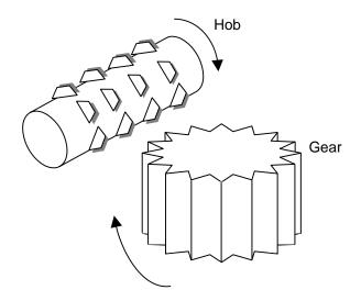
Hob axis : Rotary tool axis on which a hob is mounted. Workpiece axis : Rotary axis on which a workpiece is mounted.
