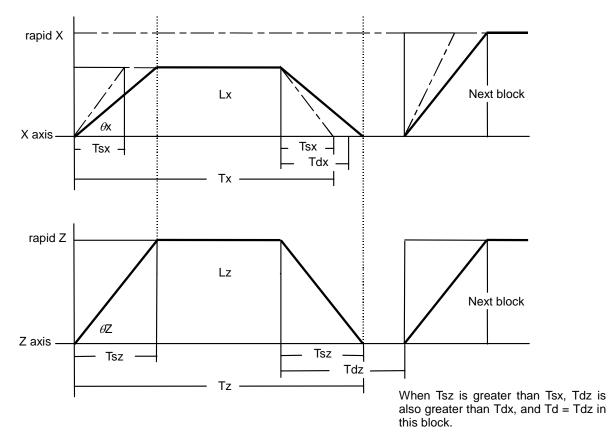
The program format of G0 (rapid traverse command) when rapid traverse constant inclination acceleration/deceleration are executed is the same as when this function is invalid (time constant acceleration/deceleration).
