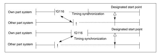
(c) When the start point designated by G116 is not on the next block movement path of the own part system, the other part system starts once the own part system has reached each start point coordinate position.
