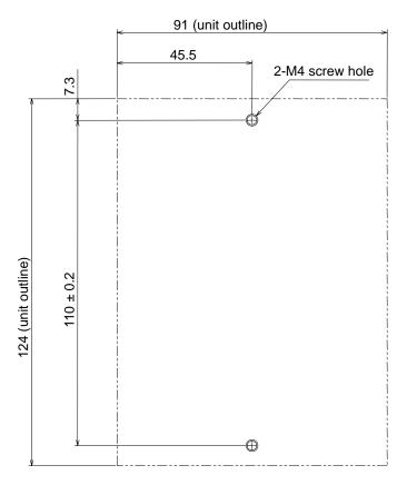
(Note) When mounting the hard disk unit, face the cable lead-out side directly straight up, and mount within ±15°.
