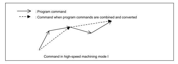
(2) Override, maximum cutting speed clamp, single block operation, dry run, manual interruption, graphic trace and high-accuracy control mode are valid even during the high-speed machining mode I.
