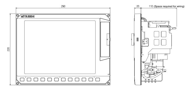
(Note) The space of 30mm or more should be provided above the display unit for maintenance.
