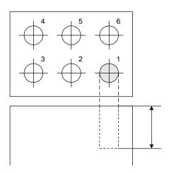
Verification stop is executed when drilling of one hole is completed (N100 block is completed) as shown on the left.
