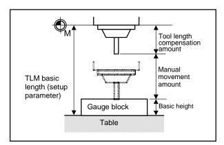
If the height axis designation parameter is ON, the axis designated for plane selection basic axis K is the axis targeted for measurement as the height axis.
