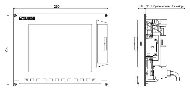
(Note 1) The above side view shows the state with the control unit mounted.
