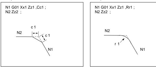
(Note 1) If a corner chamfering or corner R command is issued specifying a length longer than the N1 or N2 block, a program error occurs.
