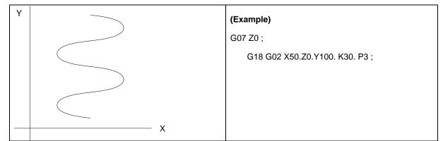
(Note) In order to perform hypothetical axis interpolation, helical interpolation must be added.
