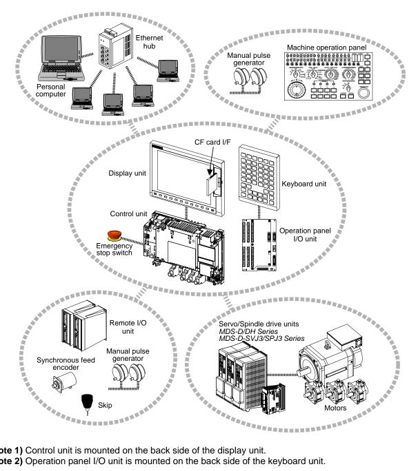
(Note 1) Control unit is mounted on the back side of the display unit. (Note 2) Operation panel I/O unit is mounted on the back side of the keyboard unit.
