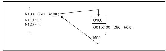
In either example 1 or 2, after the N100 cycle is executed, the N110 block is executed.
