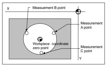
To set the workpiece coordinate offset, the position X and Y of the measurement A point are measured, and the measured values are set in the measurement A point. In the same manner as the measurement A point, the measurement B point and then C point are measured and set. The hole center coordinate is calculated by setting the workpiece coordinate system after setting three points, and the calculated result is set in the workpiece coordinate offset.
