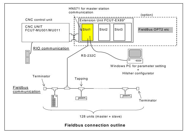
Parameters for the communication control unit installed in HN571 must be set with Hilsher configurator. Refer to the Hilsher instruction manual.
