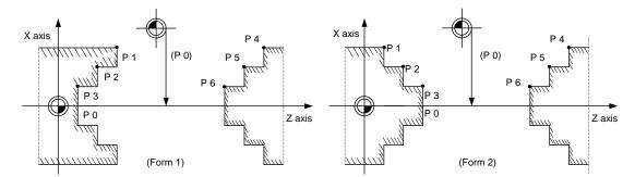
The chuck barrier and tailstock barrier are both set with the machine coordinate by inputting one set of three-point data in the parameter. Points P1, P2 and P3 are the chuck barrier, and points P4, P5 and P6 are the tailstock barrier. The X axis is set with the coordinate position (radius value) from the workpiece center, and the Z axis is set with the basic machine coordinate system coordinate.
