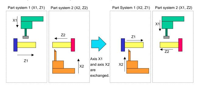
Mixed synchronization control is switched from ON to OFF and vice versa using a PLC signal.
