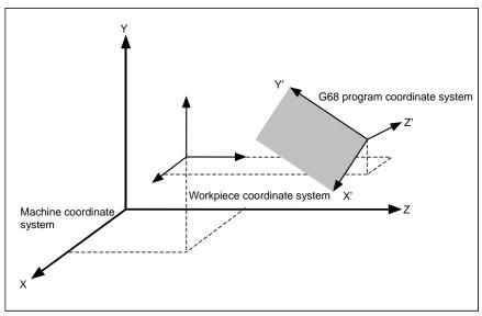
When the G68 command is issued, the zero point is shifted by the command value (x, y, z) in respect to the current local coordinate system. A new G68 program coordinate system rotated by the designated rotation angle r in respect to the commanded rotation center direction (i, j, k) is created.
