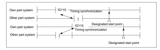
(c) When the start point designated by G115 is not on the next block movement path of the other part system, the own part system starts once the other part system has reached each start point axis coordinate position.
