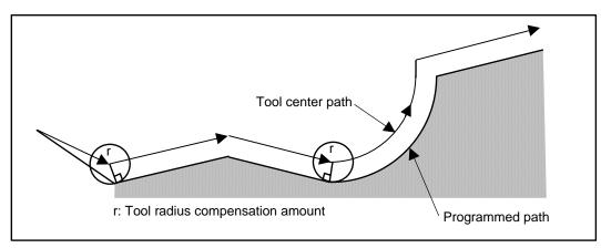
The tool radius compensation command controls the compensation from that block in which G41 or G42 is commanded. In the tool radius compensation mode, the program is read up to five blocks ahead including blocks with no movement, and interference check using tool radius is conducted up to three blocks ahead in any of those blocks with movement.
