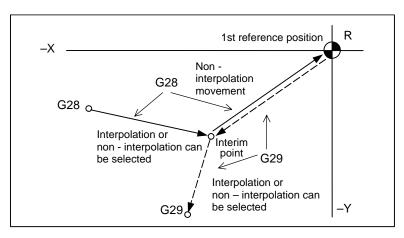
If the position detector is for the incremental detection system, the first reference position return for the first time after the NC power has been turned ON will be the dog-type. However, whether the second and subsequent returns are to be the dog type or the high-speed type can be selected by designating a parameter.
