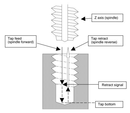
This function can be used when the machining was interrupted upon reset, emergency stop or power OFF during tapping cycle.
