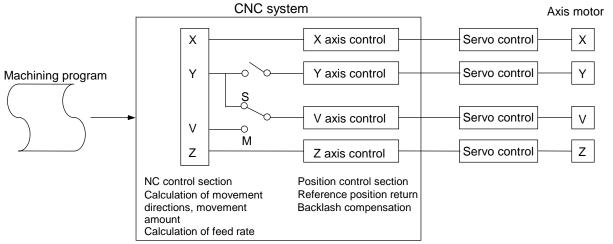
Even during independent operation, pitch error compensation, backlash compensation and external machine coordinate compensation are performed independently for each master axis and slave axis. Designation/cancellation of independent operation is executed at "all axes in-position".
