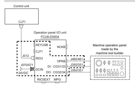
2 General Connection Diagram (M800VS/M80V Series)
