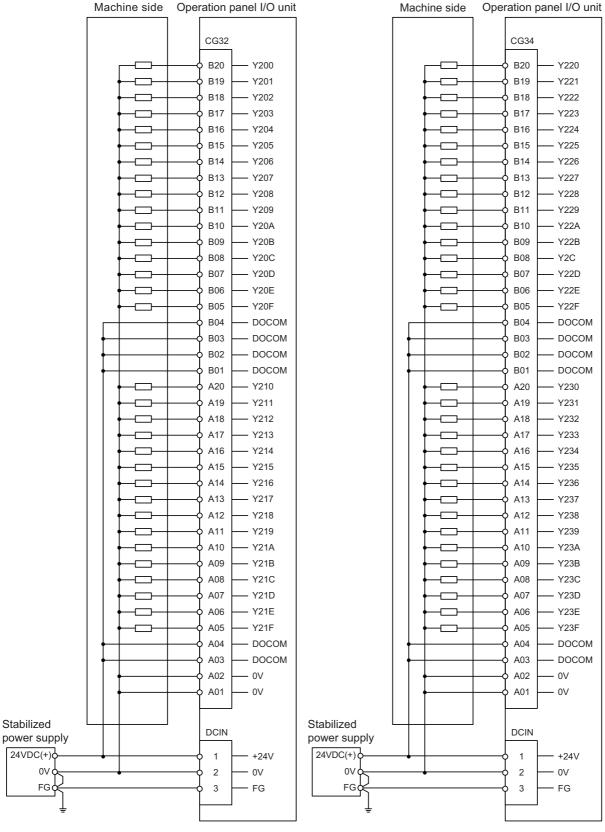
For connection details, refer to the descriptions on machine output connector pin assignment in "(2) Machine signal output (CG32)" and "(4) Machine signal output (CG34)" of "4.9 Operation Panel I/O Unit".
