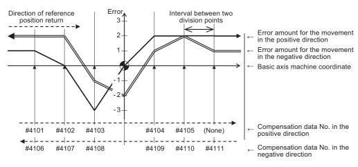
Bidirectional pitch error having odd number of compensation points (linear axis)
