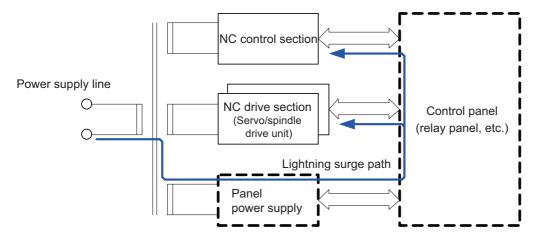
Path of damage caused by lightning surge
