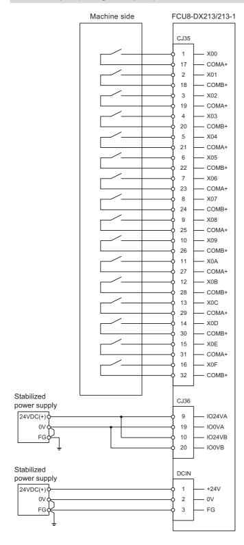
11.7 Connecting with Machine Control Signal (FCU8-DX213/FCU8-DX213-1/FCU8-DX654/FCU8-DX654-1)
