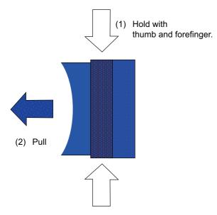
(d) For screw locking connectors, loosen the two locking screws and pull out the connector.
