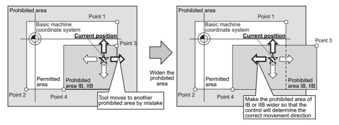
(5) As illustrated below, when stored stroke limit IB and IIB are used together, tool movement may be disabled entirely if the tool enters the overlap of the two prohibited areas. To prevent this, configure the prohibited areas of stored stroke limit IB and IIB so as not to overlap with each other. (If misconfiguration results in the tool entering the overlap of the two prohibited areas, disable stored stroke limit IIB to move the tool.)
