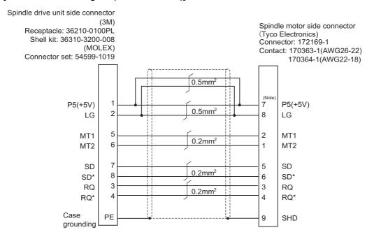
(Note) For the pin "7" or "8", use the contact "170364-1". For the other pins, use the contact "170363-1".
