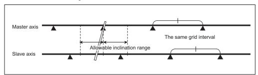
When the procedure on the next page is performed and the reference position adjustment value is other than "0", the remaining distance of the slave axis is compensated by the reference position adjustment value in step (5). Therefore, when starting position alignment after balancing, set the reference position adjustment value to "0".
