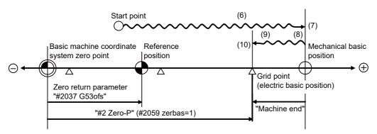
• (6) to (10) in this diagram indicate steps of the operation procedure.
