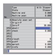
(7) Press the axis against the machine end stopper.
