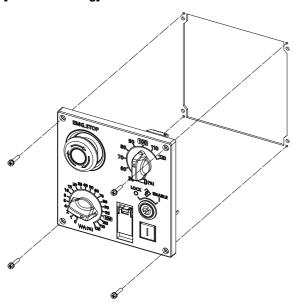
Fixing screw: Cheese head screw M3 (4 pieces) (Fixing screws are provided with the unit.)
