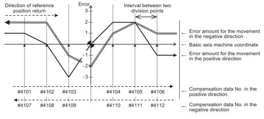
Bidirectional pitch error (linear axis)
