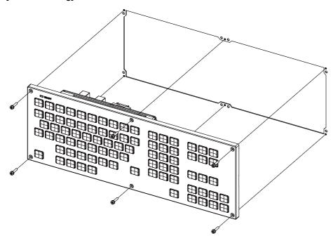
Fixing screw: Cheese head screw M3 (6 pieces) (Fixing screws are provided with the unit.)
