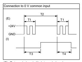
(E): External signal, (I): Internal signal
