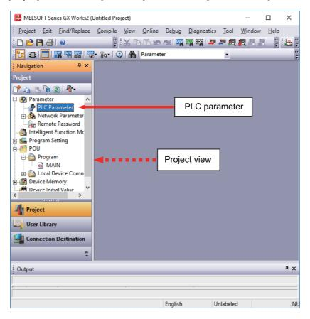
The above operation opens the following parameter setting screen. Tab names in red indicate that the initial values are set.
