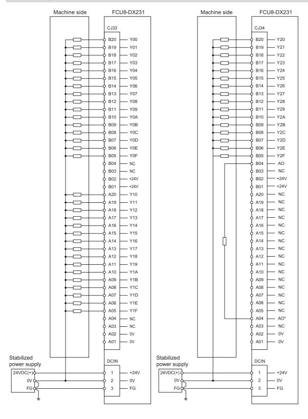
11.7 Connecting with Machine Control Signal (FCU8-DX213/FCU8-DX213-1/FCU8-DX654/FCU8-DX654-1)
