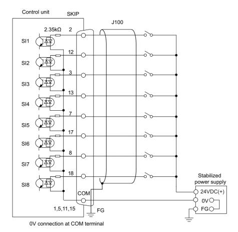
7.9 Connecting with Skip Signal (Sensor)
