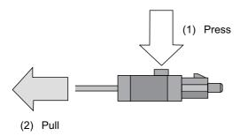
(f) For Ethernet connectors, hold down the locking tab and pull out the connector.
