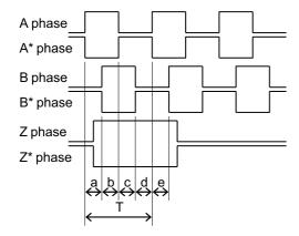
a, b, c, d and e: A phase or B phase rising edge (falling edge) phase difference =  $T/4 \pm T/10$
