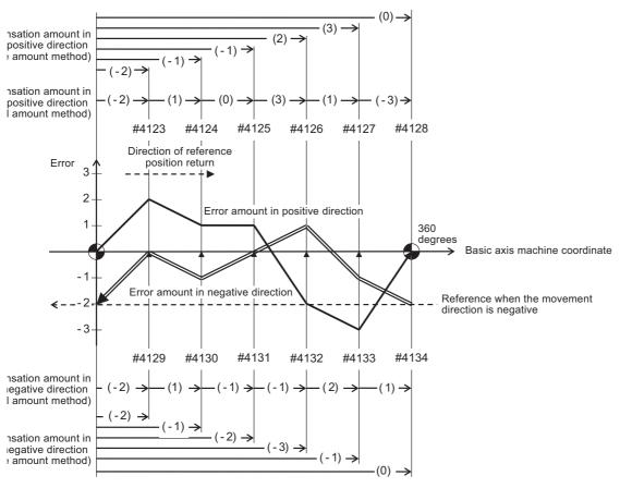
Bidirectional pitch error (rotary axis)
