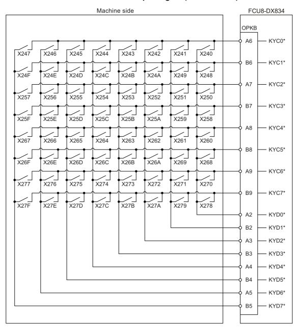
For connection details, refer to the descriptions on machine output connector pin assignment in "(15) OPKB (Scan input, Scan output)" of "4.9 Operation Panel I/O Unit".
