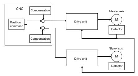
The "compensation" in the figures for position command synchronous control, speed command synchronous control, and current command synchronous control refers collectively to the pitch error compensation, thermal expansion compensation, backlash compensation, and external machine coordinate compensation.
