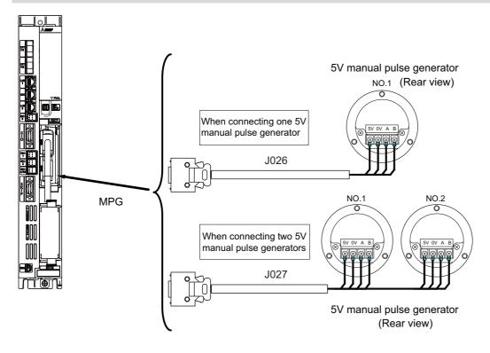
7.11 Connecting Device via Function Expansion Unit
