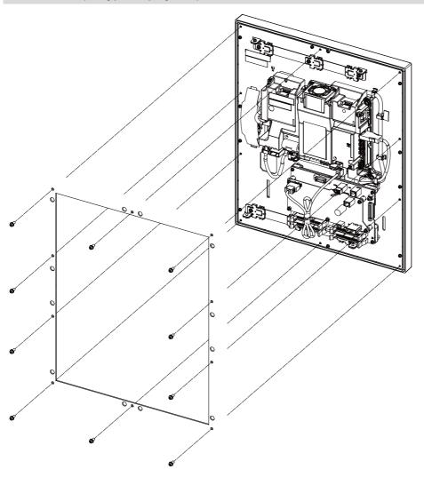
Fixing screw: Use M4  $\times$  10 with spring washer and plain washer (10 screws).
