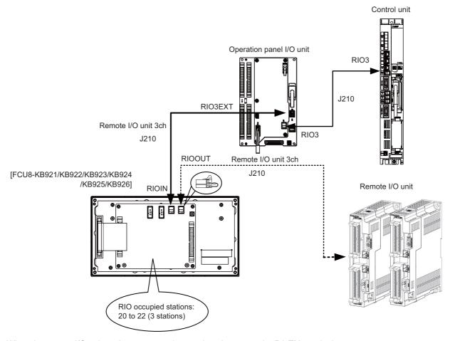
When the remote I/O unit on the next stage is not relayed, connect the R2-TM terminal.
