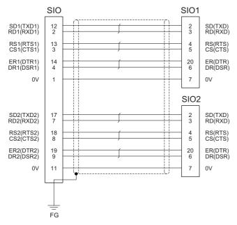
Connector: 10120-3000PE Case: 10320-52F0-008 Manufacturer: 3M Wire material: 2464C BIOS-CL3-26 07P Manufacturer: Bando Electric Wire
