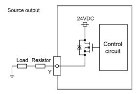
• Always keep the total sum of output current of each Y00 to Y07, Y08 to Y0F, Y10 to Y17, Y18 to Y1F, Y20 to Y27, and Y28 to Y2F less than 0.8A.
