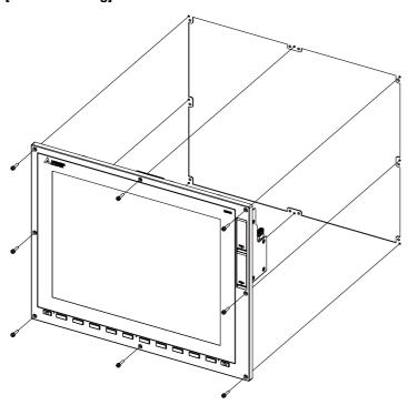
Fixing screw: Cheese head screw M3 (8 pieces) (Fixing screws are provided with the unit.)
