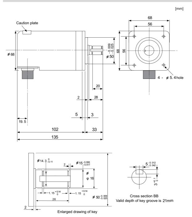
4 General Specifications 4.14 Synchronous Feed Encoder
