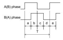
a, b, c, d and e: A phase or B phase rising edge (falling edge) phase difference =  $T/4 \pm T/10$  T: A or B phase cycle
