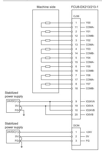
11.7 Connecting with Machine Control Signal (FCU8-DX213/FCU8-DX213-1/FCU8-DX654/FCU8-DX654-1)
