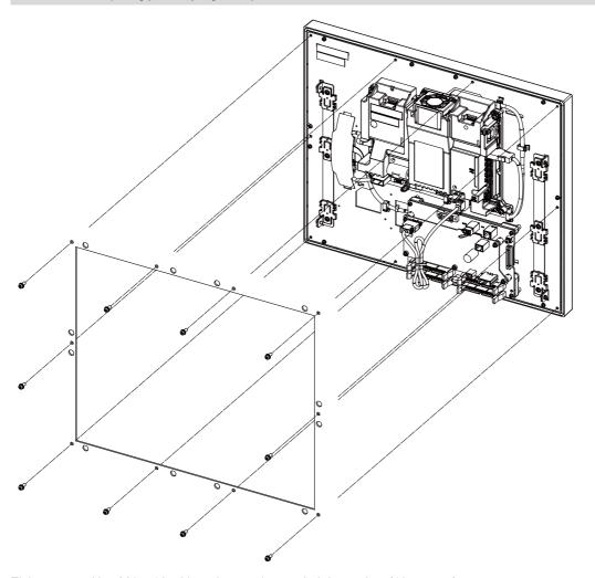
Fixing screw: Use M4  $\times$  10 with spring washer and plain washer (10 screws).
