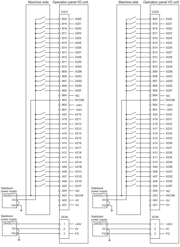
For connection details, refer to the descriptions on machine input connector pin assignment in "(1) Machine signal input (CG31)" and "(3) Machine signal input (CG33)" of "4.9 Operation Panel I/O Unit".
