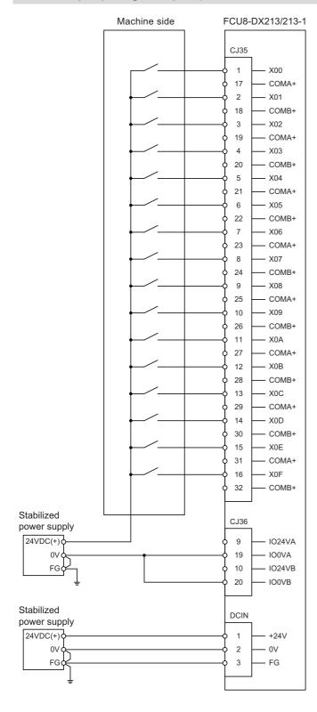
11.7 Connecting with Machine Control Signal (FCU8-DX213/FCU8-DX213-1/FCU8-DX654/FCU8-DX654-1)
