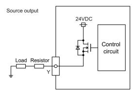
• Always keep the total sum of output current of each Y00/Y02/Y04/Y06 and Y01/Y03/Y05/Y07 less than 4A.
