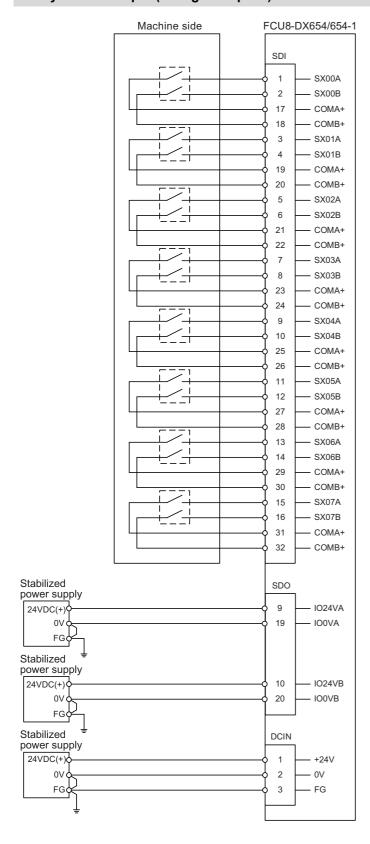
11.7 Connecting with Machine Control Signal (FCU8-DX213/FCU8-DX213-1/FCU8-DX654/FCU8-DX654-1)
