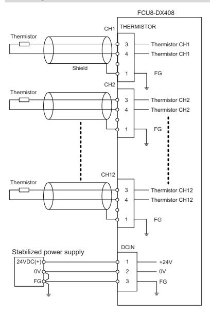
11.11 Connecting with Multi-analog Input Signal (FCU8-DX409)
