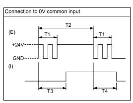
(E): External signal, (I): Internal signal
