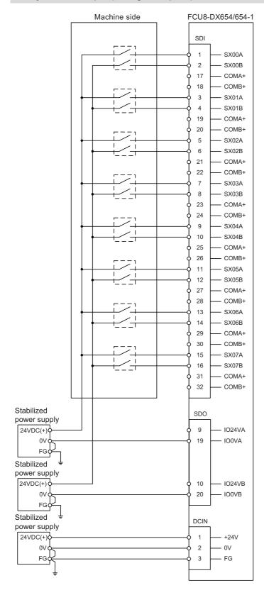
11.7 Connecting with Machine Control Signal (FCU8-DX213/FCU8-DX213-1/FCU8-DX654/FCU8-DX654-1)
