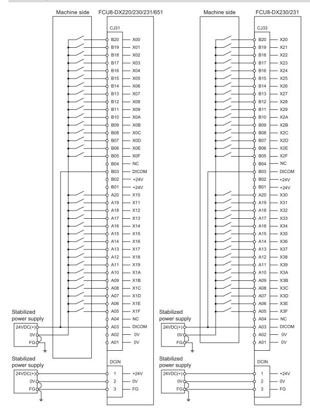
11.6 Connecting with Machine Control Signal (FCU8-DX220/FCU8-DX230/FCU8-DX231/FCU8-DX651)
