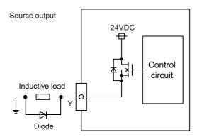
When the rush current exceeds the maximum output current indicated previously, always connect a protective resistor serially to the load to suppress rush currents. Make sure that the current is less than the maximum output current including the momentary current.
