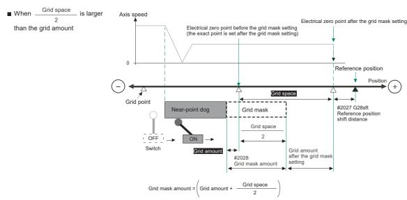
24.2 Adjustment of Reference Position Return in Relative Position Detection System
