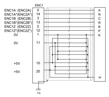
[ENC1] Plug: 10120-3000VL Shell: 10320-52F0-008 Manufacturer: 3M Wire material: UL1061-2464 AWG24 × 12P Manufacturer: Oki Electric Cable
