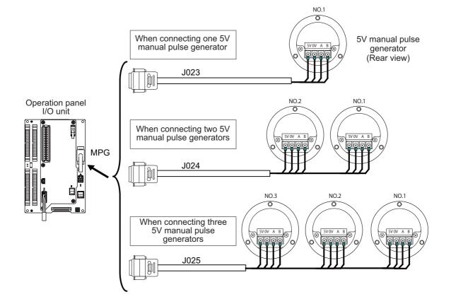
10.9 Connecting with Manual Pulse Generator (MPG)
