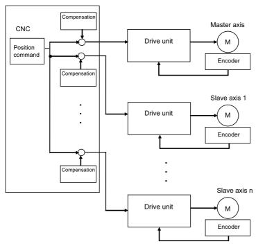
The "compensation" in the figure refers collectively to the pitch error compensation, thermal expansion compensation, backlash compensation, and external machine coordinate compensation. Even under the multiple-axis synchronization control, the compensation is performed independently for each axis.
