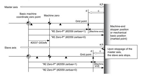
The following is the operation example of stopper method when the slave axis reaches the stopper first:
