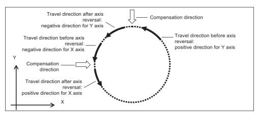
When a negative value is set as a compensation amount, compensation is performed in the travel direction of the axis before axis reversal.
