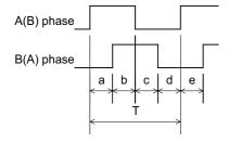
a, b, c, d and e: A phase or B phase rising edge (falling edge) phase difference =  $T/4 \pm T/10$
