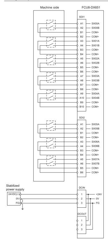
11.8 Connecting with Safety Machine Control Signal (FCU8-DX651)
