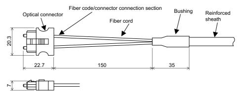
To ensure the system performance and reliability, purchase the optical communication cable from Mitsubishi. A machining drawing is given in "Cable" as reference, but the purchased optical communication cable cannot be cut or connected by the machine tool builder.
