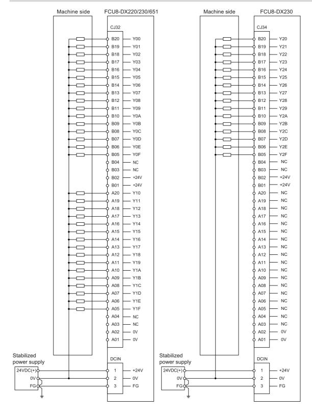
11.6 Connecting with Machine Control Signal (FCU8-DX220/FCU8-DX230/FCU8-DX231/FCU8-DX651)
