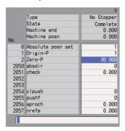
The zero point initial setting is now complete. After initializing all axes, turn the power OFF and ON.
