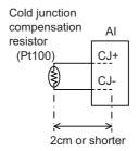
Set the lead length 2cm or shorter including the length to insert to AI connector. (As a guide)
