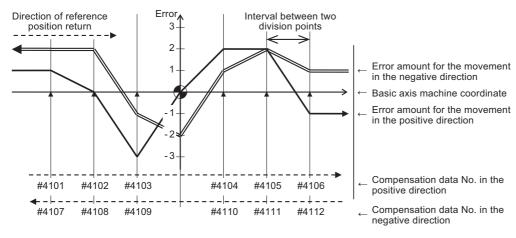
Bidirectional pitch error (linear axis)
