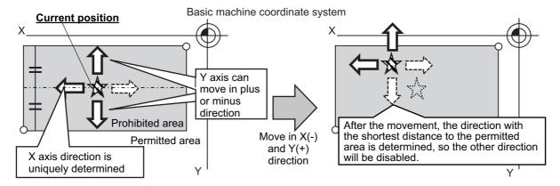
(4) If this function is used together with the stored stroke limit function that does not support this function, the tool may be allowed to move towards the prohibited area of the combined stored stroke limit function, as illustrated below. To prevent this, it is recommended to set the ranges of stored stroke limit IB and IIB to be large enough.
