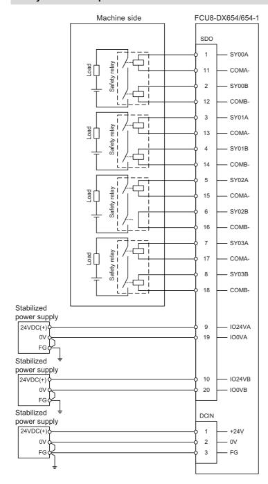
11.8 Connecting with Safety Machine Control Signal (FCU8-DX651)
