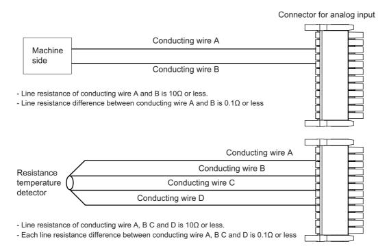
11.11 Connecting with Multi-analog Input Signal (FCU8-DX409)
