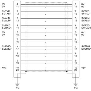
[CN4, CN9] Plug: 10120-3000PE Shell: 10320-52F0-008 Manufacturer: 3M Wire material: UL20276 AWG28 × 10P Manufacturer: Toyokuni Electric Plug: 10120-3000PE Shell: 10320-52F0-008 Manufacturer: 3M
