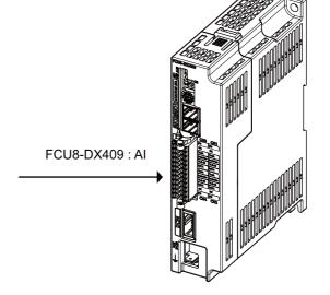
Maximum cable length is 50 m. Line resistance is 10  $\Omega$  or less, and line resistance difference is 0.1  $\Omega$  or less (see below).
