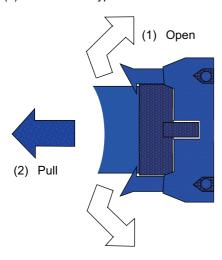
(c) For flat cable type connector without latches, hold the connector with a thumb and forefinger and pull the connector off.
