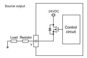
• Always keep the total sum of output current of each SY00A to SY03A, and SY00B to SY03B less than 4A.
