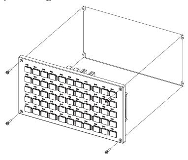
Fixing screw: Cheese head screw M3 (4 pieces) (Fixing screws are provided with the unit.)
