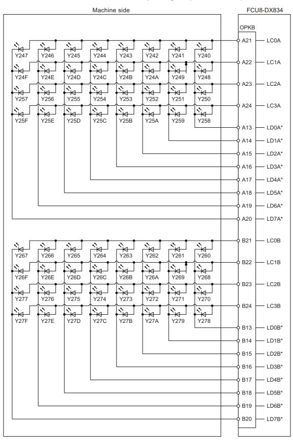
For connection details, refer to the descriptions on machine output connector pin assignment in "(15) OPKB (Scan input, Scan output)" of "4.9 Operation Panel I/O Unit".
