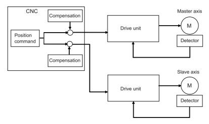
The position command synchronous control has the following configuration:
