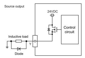
When the rush current exceeds the maximum output current indicated previously, always connect a protective resistor serially to the load to suppress rush currents. Make sure that the current is less than the maximum output current including the momentary current.
