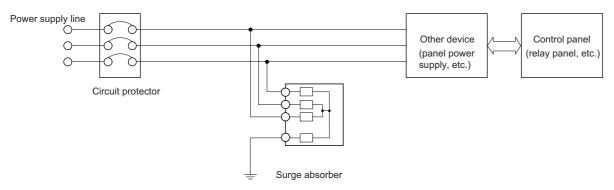
Lightning surge countermeasure for three-phase power supply line
