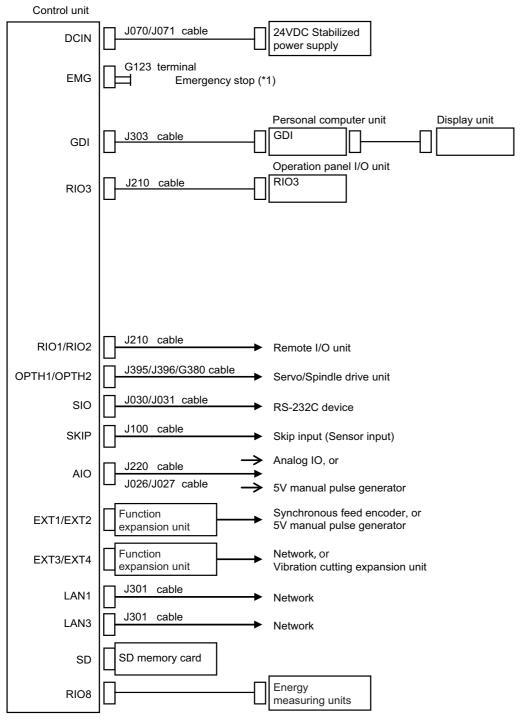
(\*1) Use when installing an emergency stop switch in the electric cabinet. (Connection cable: J120 cable) When this connector is not used, connect a terminator connector (G123 cable). G123 terminal cable comes with the control unit.
