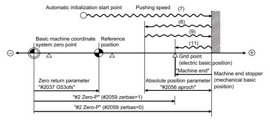
• (7) to (11) in this diagram indicate steps of the operation procedure.
