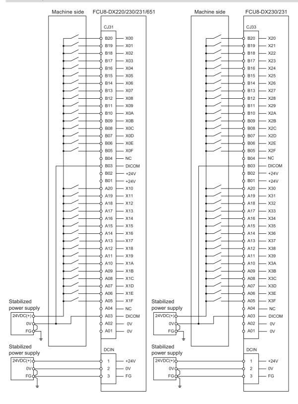
11.6 Connecting with Machine Control Signal (FCU8-DX220/FCU8-DX230/FCU8-DX231/FCU8-DX651)
