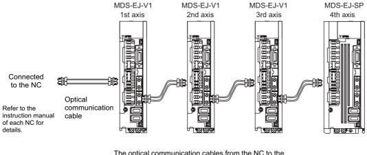
The optical communication cables from the NC to the final drive unit must be within 30m.
