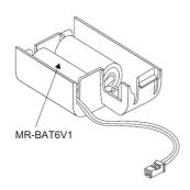
Replace the built-in battery with a new battery for MR-BAT6V1.
