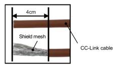
(2) Isolate the shield mesh and the wires coverd with shield tape. Remove the shield tape from wires.
