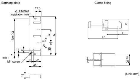
(Note 1) Screw hole for wiring to earthing plate in cabinet. (Note 2) The earthing plate thickness is 1.6mm.
