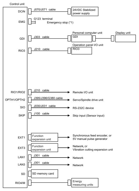
(\*1) Use when installing an emergency stop switch in the electric cabinet. (Connection cable: J120 cable) When this connector is not used, connect a terminator connector (G123 cable). G123 terminal cable comes with the control unit.
