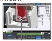
Machine interference is highlighted in color to be spotted easily
