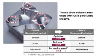
"Cutting load control" automatically controls cutting load, leading to longer tool life and shorter cycle time.
