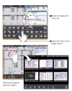
Usability of the M800/M80 Series has further evolved! Multi-touch gestures enable smarter operations, such as: Pinch-in/pinch-out in program display area to change text size
