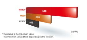
With improved hardware optimized for CNC, the dedicated CPU significantly improves fine segment processing capability.
