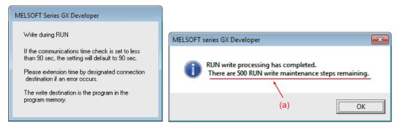
Ignore the message "There are xxx RUN write maintenance steps remaining." indicated by (a) in the completion dialog box. CNC does not use such kind of steps.
