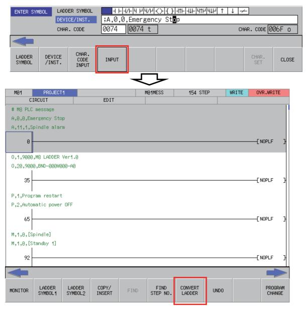
It turns to an unconverted ladder. Press the [CONVERT LADDER] menu to determine the edit contents. For details of conversion, refer to "6.13.2.7 Converting Programs".
