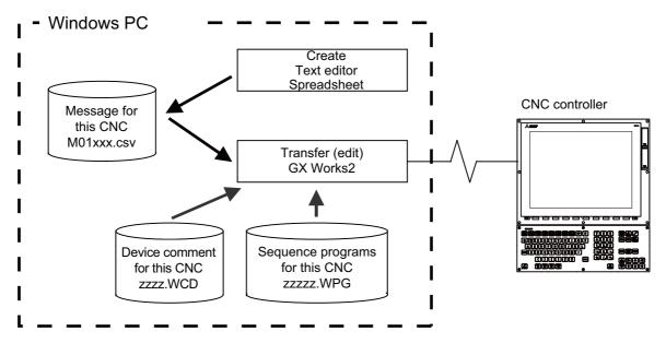
(Note) In GX Works2, only CSV files can be read. Unlike GX Developer, TXT files cannot be read. CSV files of GX Works2 projects with label settings cannot be read, in which case, PLC message can only be developed by inputting messages directly from GX Works2.
