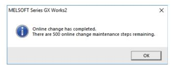
Ignore the message "There are xxx RUN write maintenance steps remaining." indicated by (a) in the completion dialog box. CNC does not use such kind of steps.
