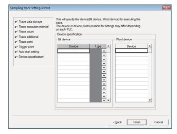
At wizard setting/execution - Sampling trace setting wizard - Trigger point setting - Device setting screen
