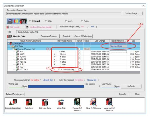
In the above screen example, adjust the size of the sequence program so that the total number of steps at execution (37) indicated in (c) is smaller than the denominator: the maximum size (1032128) of the execution area.
