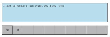
2. Pressing the [YES] menu key closes the message screen and resets all files to the password not set state (password locked state). The cancel password popup screen closes and the PLC data stored in the NC is retrieved again.
