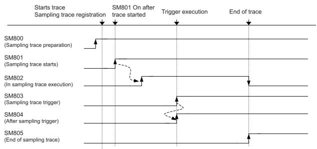
\*SM800 automatically turns ON when sampling trace preparation is done.
