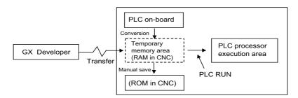
When a sequence program is transfered from the temporary storage area to the execution area, the program execution format is converted to that of the sequence program. Although the execution area of the PLC processor has twice the capacity of the temporary storage area, PLC cannot be executed if the capacity exceeds the allowable range.
