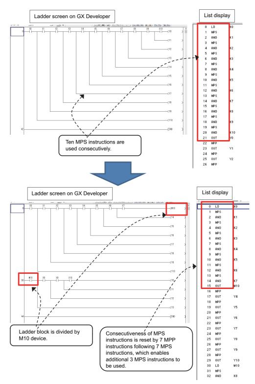
Set NC parameter "#6456 bit0" to "1" to display an error dialog on GX Developer when sequence programs that do not conform to restrictions (1) and (2) are written, and thereby prevent PLC from becoming RUN status. When an error dialog is displayed, use the above substitute ladder.
