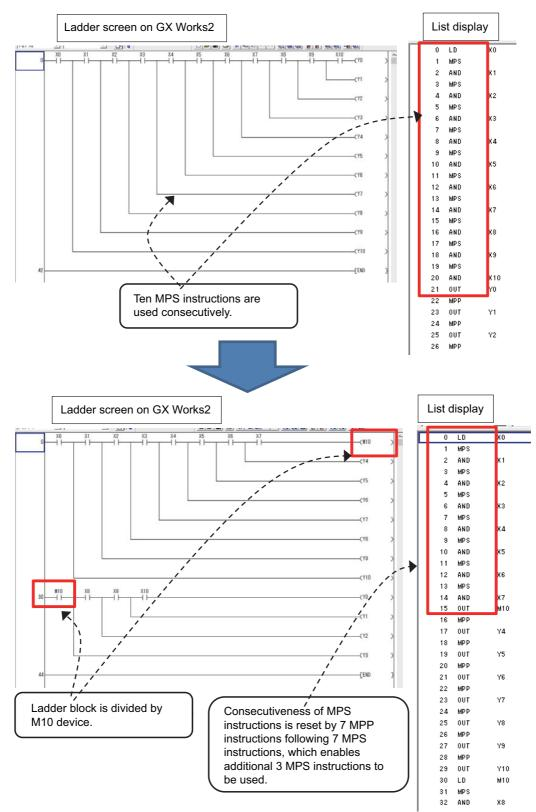
Set the NC parameter "#6456/bit0" to "1" to display an error dialog on GX Works2 when sequence programs that do not conform to restrictions (1) and (2) are written, and thereby prevent PLC from becoming RUN status. When an error dialog is displayed, use the above substitute ladder.
