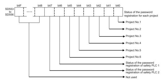
The values of the special registers change depending on the status of the password registration for stored file. However, the target file of the register and condition to change the value differ for the respective registers. For details, refer to the following table.
