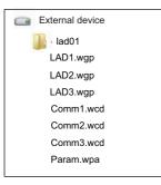
\* In this method, the temporary work directory "WorkTemp" is created when updating the PLC version directly under the "ladXX" directory and is deleted after the update.
