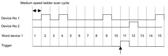
Trigger execution timing (Scan when "word device 1=11" has been established.
