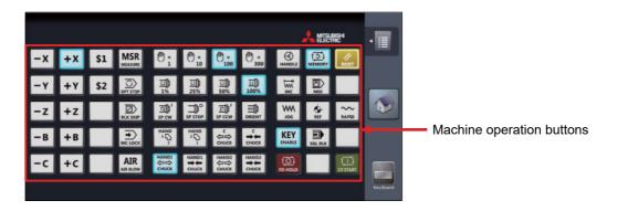
Pressing each machine operation button turns ON the PLC input signal which has been assigned to the button. When the PLC output signal which has been assigned to the button becomes ON state, the button color turns to that indicates ON state.
