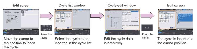
Once you insert a cycle block, you can edit it directly on the program edit screen, or re-edit it in the cycle edit window if the cycle format is not changed.
