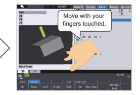
(Example) Rotate about the vertical axis
