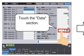
The parameter screen is being displayed (the cursor position is at #1026).
