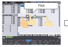
A workpiece coordinate system offset (G54-G56) is being displayed.
