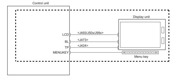
2.4 Connecting an Operation Panel I/O Unit (FCU8-DX834)
