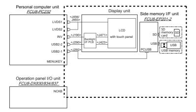
• The personal computer unit is installed on the back of the display unit.
