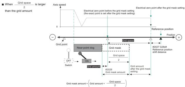
(6) Set the determined grid mask amount for "#2028 grmask" of the [ZERO-RTN PARAM] screen.
