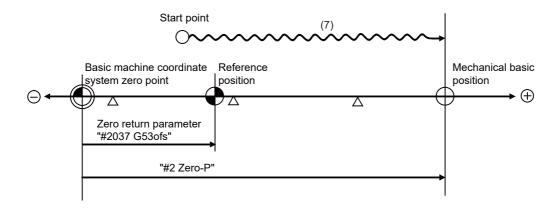
(Note 1) To change just the basic machine coordinate zero point, set "#0 Absolute posn set" and "#2 Zero-P", and then turn the power OFF and ON.
