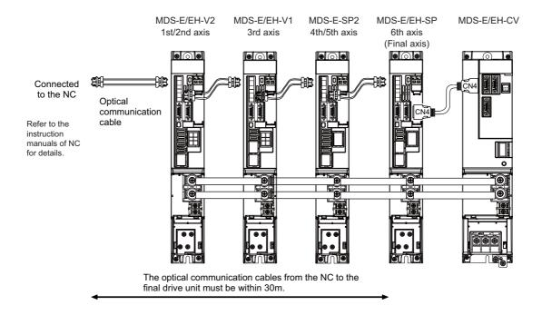
Connection when using one power supply unit
