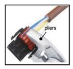
(5) Insert the CC-Link cable into the connector of CC-Link unit.
