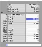
The zero point initial setting is now complete. After initializing all axes, turn the power OFF and ON.
