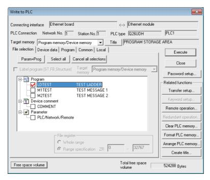
(Note) Only "Program memory/Device memory" is valid for "Target memory".Do not carry out the setting for other tabs than [File selection] ([Device data], [Program], [Common], [Local]).
