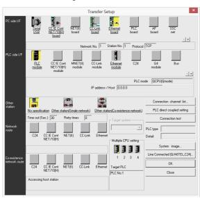
(3) Press the [Connection test] button after completing the setting.
