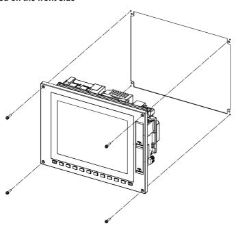
Fixing screw: Cheese head screw M3 (4 pcs). (Fixing screws are provided with the unit.)
