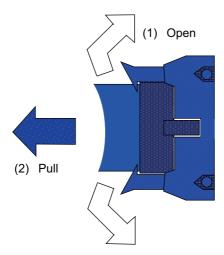
(c) For a flat cable type connector without latches, hold the connector with a thumb and forefinger, and pull the connector off.
