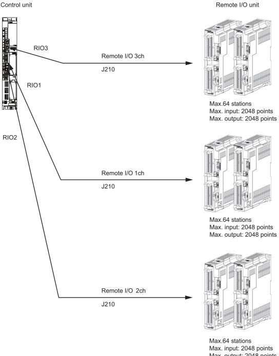
Max. output: 2048 points (Note) Connect the J210 cable to the RIO1, RIO2, or RIO3 connector of the control unit.
