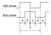
a.b.c.d.e: A phase or B phase rising edge (falling edge) phase difference =  $T/4 \pm T/10$  T: A or B phase cycle
