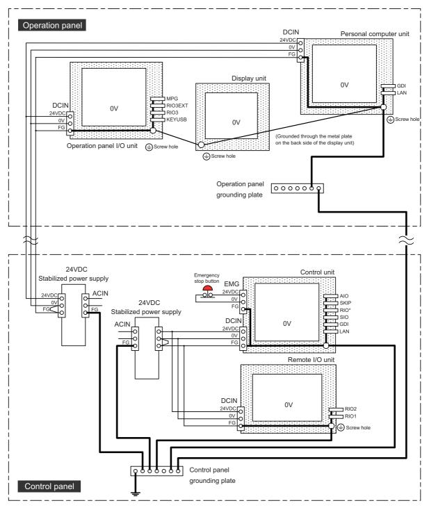
: Indicates that the metal case of connector is connected to FG (a) according to the pattern on PCB.
