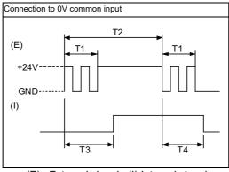
(E): External signal, (I):Internal signal
