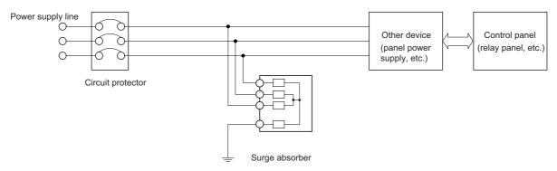
Lightning surge countermeasure for three-phase power supply line
