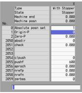
(6) [When the parameter "#2059 zerbas" is set to "0"] Set "Zero-P" here. (\*2) Move the cursor to "Zero-P" with the [↑] and [↓] keys. Input the distance from the basic machine coordinate zero point to the basic position in the input area, and press the [INPUT] key.
