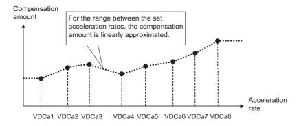
The variable torsion compensation is invalid on the axis where "0" is set to the acceleration rate of the 1st parameter. When the size correlation of the acceleration rates is incorrectly set from the 1st to 8th parameters, the incorrectly set parameter and the subsequent parameters are invalid.
