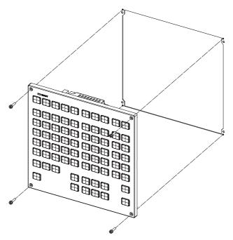
Fixing screw: Cheese head screw M3 (4 pcs). (Fixing screws are provided with the unit.)
