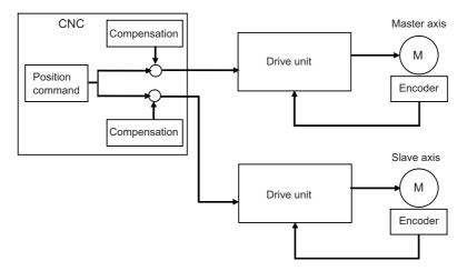
The position command synchronous control has the following configuration:
