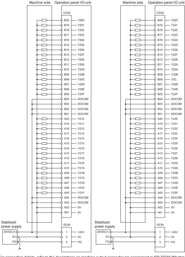
For connection details, refer to the descriptions on machine output connector pin assignment in "(2) CG32 (Machine signal output)" or "(4) CG34 (Machine signal output)" of "General Specifications: Operation Panel I/O Unit".
