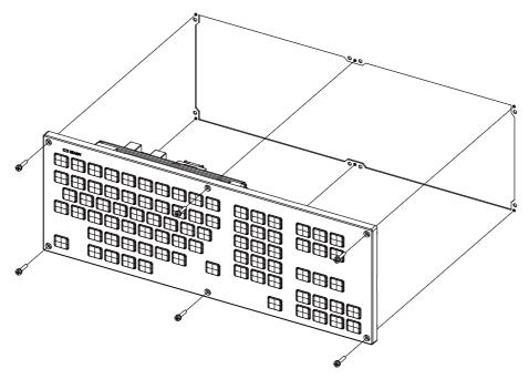
Fixing screw: Cheese head screw M3 (6 pcs). (Fixing screws are provided with the unit.)
