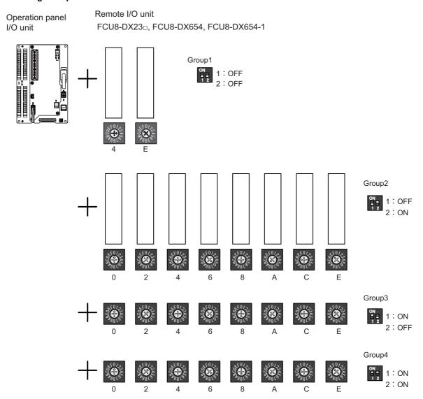
(Note) The maximum connectable number of remote I/O units is 32.
