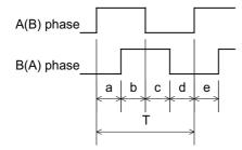
a.b.c.d.e: A phase or B phase rising edge (falling edge) phase difference =  $T/4 \pm T/10$  T: A or B phase cycle
