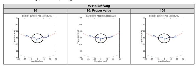
(Note) Even though #2111 is set to "1", if any of #2112, #2113, or #2115 is set to "0", the quadrant projection compensation is invalid.
