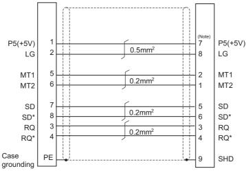
(Note) For the pin "7" or "8", use the contact "170364-1". For the other pins, use the contact "170363-1".
