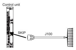
(Note) Connecting the skip signal cable to a wrong connector causes a damage on the control unit when turning ON the skip signal power supply. Confirm the wiring before turning the power ON.
