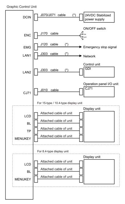
(Note 1) The section indicated with asterisk (\*) indicates cable to be wired outside the operation panel.
