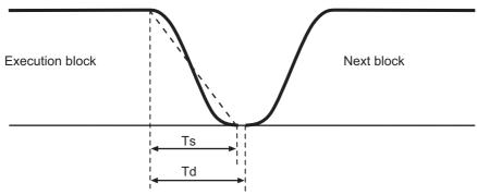
Ts : Soft acceleration/deceleration time constant Td : Deceleration check time Td = Ts +  $\alpha$ (0 to 10ms)
