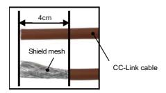
(2) Isolate the shield mesh and the wires coverd with shield tape. Remove the shield tape from wires.
