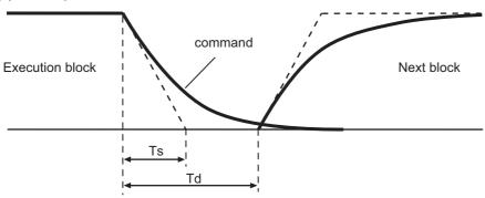
Ts: Exponential acceleration/deceleration time constant Td: Deceleration check time Td =  $Ts \times 2 + \alpha(0 \text{ to } 10 \text{ms})$
