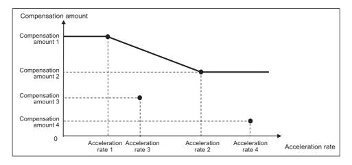
When the number of measured compensation patterns are less than four, compensation is carried out for the compensation patterns which are measured by setting "0" to acceleration rates corresponding to compensation patterns which have not been measured yet.
