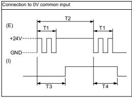
(E): External signal, (I):Internal signal
