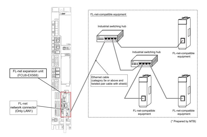
(Note 1) FL-net expansion unit is equipped with two RJ-45 connectors (LAN1 and LAN2); however, the function of FL-net is available only on LAN1. Do not connect any cable to LAN2 port.
