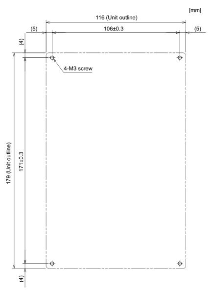
(Note) The unit thickness of the fixed part with screws is 16.6mm.Select the fixing screws having the length suitable for the thickness.
