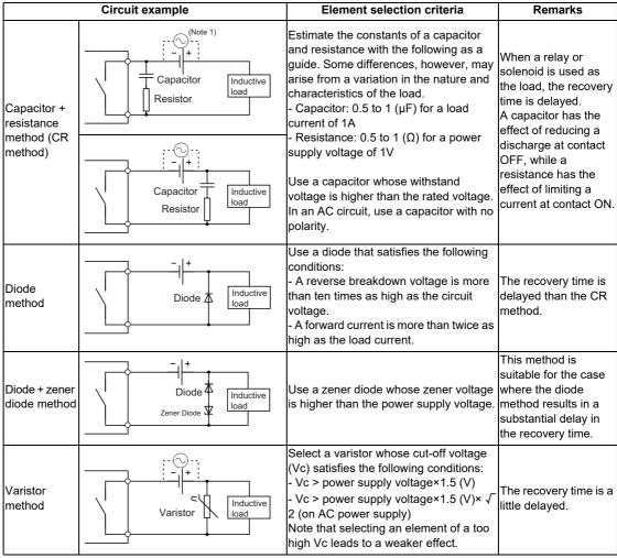
(Note 1) On AC power supply, the impedance of the CR needs to be sufficiently higher than that of the load (for preventing errors due to the leakage current of the CR).
