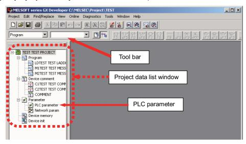
(2) Displaying the parameter setting screen Perform the following operations to display the parameter setting screen. The characters of tab in "red" show that the settings are the initial values.
