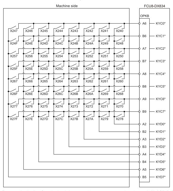
For connection details, refer to the descriptions on machine output connector pin assignment in "(15) OPKB (Scan input, Scan output)" of "General Specifications: Operation Panel I/O Unit".
