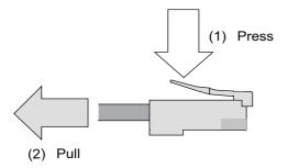
(g) For the USB connector, pull off while holding down the locked latch.
