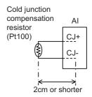
Set the lead length 2cm or shorter including the length to insert to Al connector. (As a guide)
