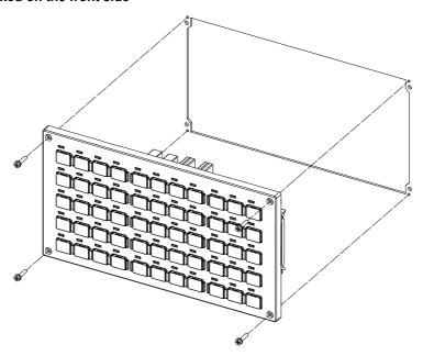
Fixing screw: Cheese head screw M3 (4 pcs). (Fixing screws are provided with the unit.)
