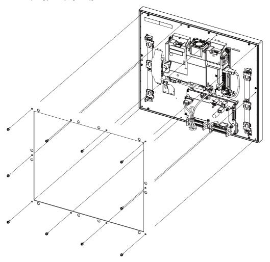
Fixing screw: Use M4×10 with spring washer and plain washer (10 screws).
