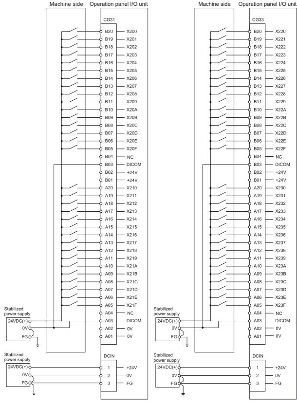
For connection details, refer to the descriptions on machine input connector pin assignment in "(1) CG31 (Machine signal input)" or "(3) CG33 (Machine signal input)" or "General Specifications: Operation Panel I/O Unit".
