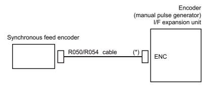
(Note 1) The section indicated with asterisk (\*) indicates cable to be wired outside the electric cabinet.
