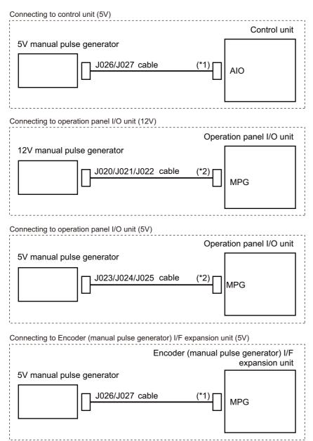
(Note 1) (\*1) in the figure indicates cable to be wired outside the electric cabinet, and (\*2) indicates cables to be wired outside the operation panel.
