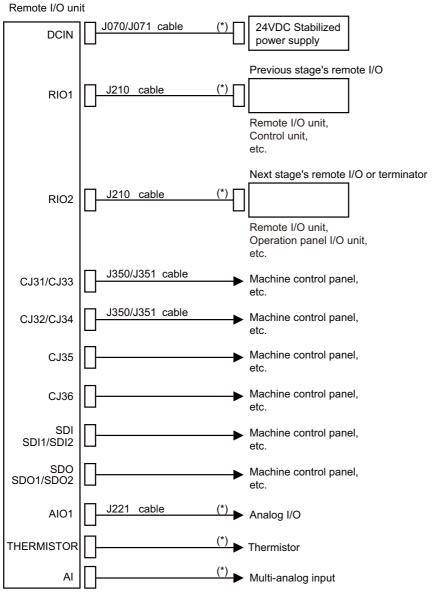
(Note 1) The mounted connector differs depending on the unit. Refer to the following chapter for which of the connector is mounted.
