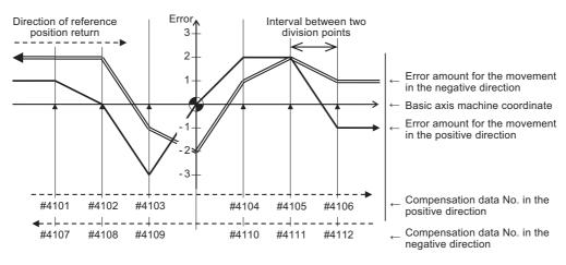
Bidirectional pitch error (linear axis)
