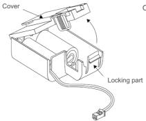
Open the cover while pushing the locking part.
