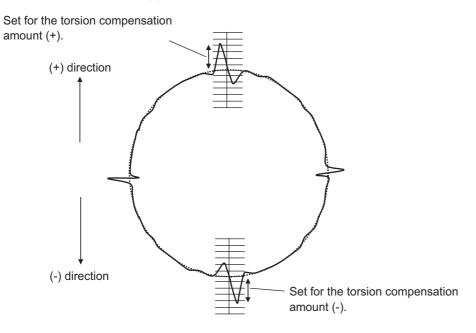
The torsion compensation amount parameters are as follows.
