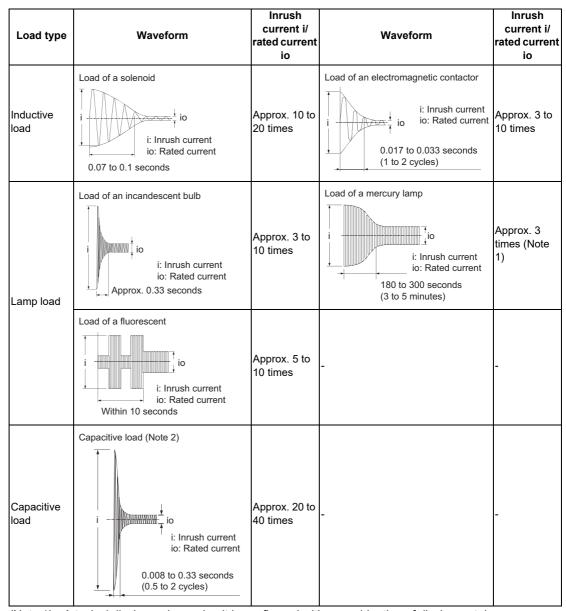
(Note 1) A typical discharge lamp circuit is configured with a combination of discharge tubes, transformers, choke coils, capacitors and others. Because of this, be especially careful of the case of a high power factor and a low power supply impedance, where the inrush current flowing into the output module can be 20 to 40 times as high as the rated current.
