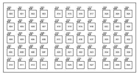
(Note 1) If the stations of machine operation panel and other remote I/O unit overlap, all the connections of the overlapping stations are invalidated and cannot be used. Stations which do not overlap can be used.
