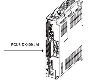
Maximum cable length is 50m. Line resistance is  $10\Omega$  or less, and line resistance difference is  $0.1\Omega$  or less (see below).
