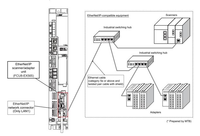
(Note 1) EtherNet/IP scanner/adapter unit is equipped with two RJ-45 connectors (LAN1 and LAN2); however, the function of EtherNet/IP is available only on LAN1. Do not connect any cable to LAN2 port.
