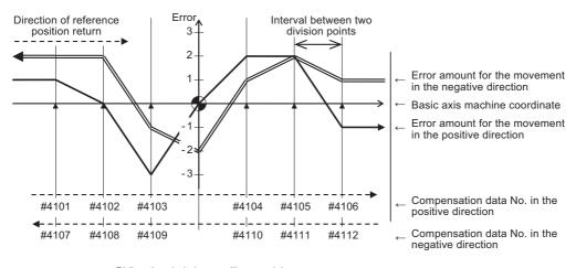
Bidirectional pitch error (linear axis)
