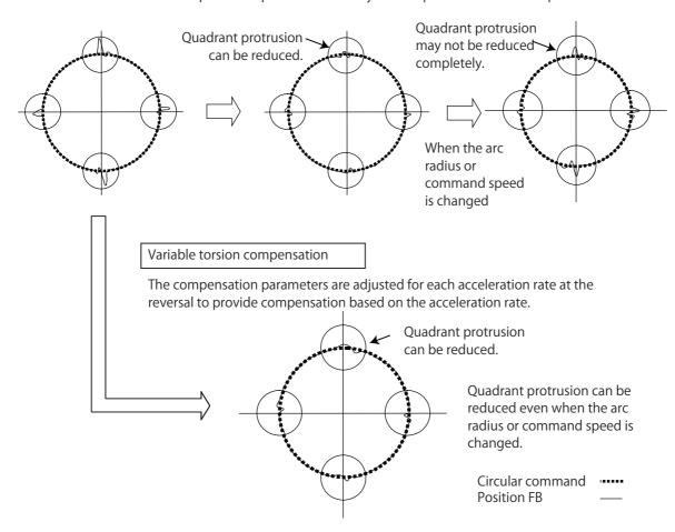
This function is valid only on the first part system. Also, this function is valid on the basic axis and the additional axis. This function is invalid on the rotary axis and spindle.
