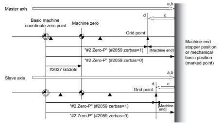
(Note) In carrying out zero point initial setting, even when one axis has stopped on a grid, the other axis keeps traveling. Thus, decelerate enough before setting.
