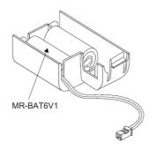
Replace the built-in battery with a new battery for MR-BAT6V1.
