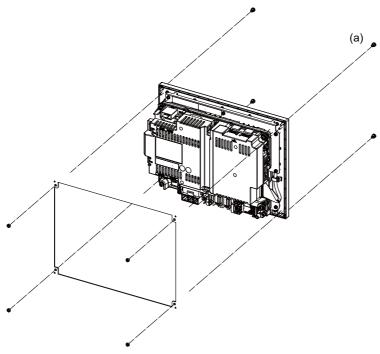
Fixture: M3 nut (4 pcs). (4 pcs of the screw caps (a) are provided with the unit.)
