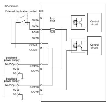
(Note) This circuit drawing is an example when two stabilized power supplies are used.
