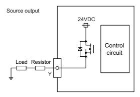
(Note 3) Always keep the total sum of output current of each Y00 to Y07, Y08 to Y0F, Y10 to Y17, Y18 to Y1F, Y20 to Y27, and Y28 to Y2F less than 0.8A.
