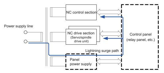
Path of damage caused by lightning surge
