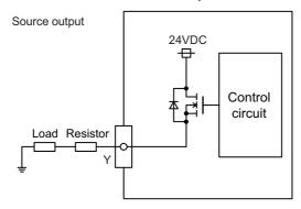
(Note 3) Total output current for each of Y00/Y02/Y04/Y06 and Y01/Y03/Y05/Y07 must be 4A or less.
