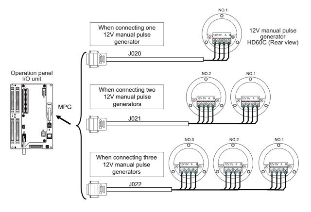
(Note 1) When selecting a manual pulse generator, make sure that its case and 0V terminal are insulated.
