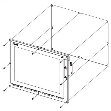
Fixing screw: Cheese head screw M3 (8pcs). (Fixing screws are provided with the unit.)
