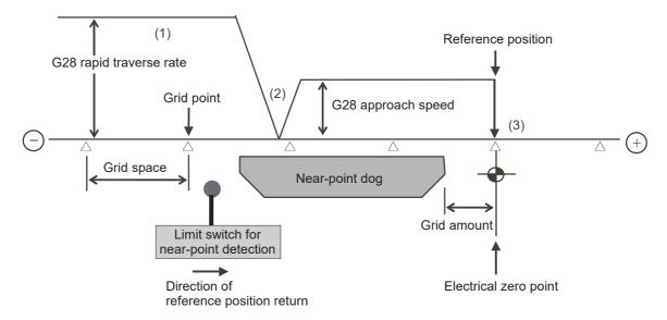
The first reference position return after turning the power ON is carried out with the dog-type reference position return. The second and following returns are carried out with either the dog-type reference position return or the high-speed reference position return, depending on the parameter.
