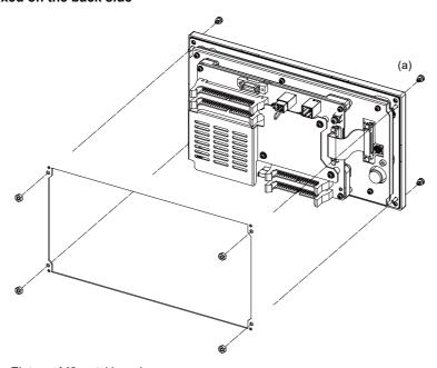
Fixture: M3 nut (4 pcs). (4 pcs of the screw caps (a) are provided with the unit.)
