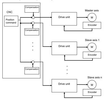
The "compensation" in the figure indicates the pitch error compensation, the thermal expansion compensation, the backlash compensation and the external machine coordinate compensation. Even under the multiple-axis synchronization control, the compensation is performed independently for each axis.
