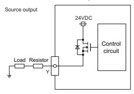
(Note 3) Total output current for each of SY00A to SY03A and SY00B to SY03B must be 4A or less.
