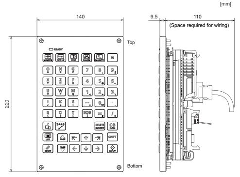
(Note) The above side view shows the state with the operation panel I/O unit mounted.
