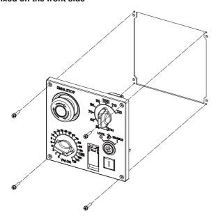
Fixing screw: Cheese head screw M3 (4 pcs). (Fixing screws are provided with the unit.)
