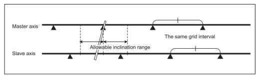
When the procedure on the next page is performed while the reference position adjustment value is other than "0", the remaining distance of the slave axis is compensated by the reference position adjustment value in step (e). Therefore, set the reference position adjustment value to "0" when starting position alignment after balancing. For speed command synchronization and current command synchronization, carry out "(2) Position alignment without using reference position adjustment value".
