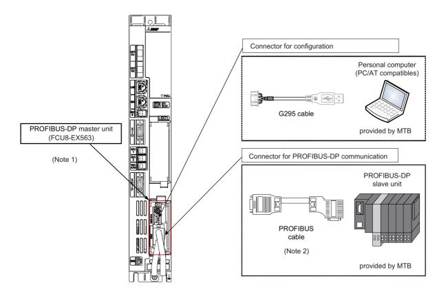
(Note 1) Use the rotary switch of PROFIBUS-DP master unit with the initial value "0".
