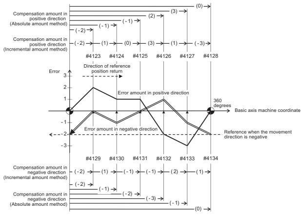
Bidirectional pitch error (rotary axis)
