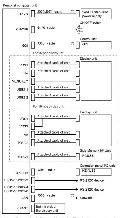
(Note 1) The section indicated with asterisk (\*) indicates cable to be wired outside the operation panel.
