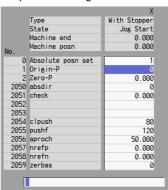
(6) [When the parameter "#2059 zerbas" is set to "0"] Set "Zero-P" here. (\*2) Move the cursor to "Zero-P" with the [↑] and [↓] keys. Input the distance from the basic machine coordinate zero point to the basic position in the input area, and
