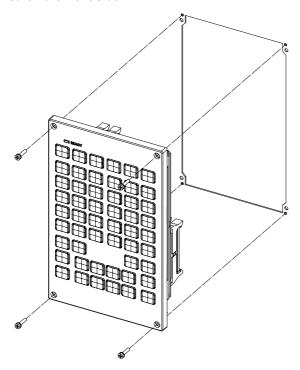
Fixing screw: Cheese head screw M3 (4 pcs). (Fixing screws are provided with the unit.)
