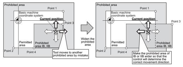
(5) As illustrated below, when stored stroke limit IB and IIB are used together, and the tool enters the overlap of the two prohibited areas, movement of the tool may be disabled. To prevent this, configure settings so that the prohibited areas of stored stroke limit IB and IIB will not overlap with each other. (If the tool has entered both prohibited areas due to an incorrect setting, disable stored stroke limit IIB to move the tool.)
