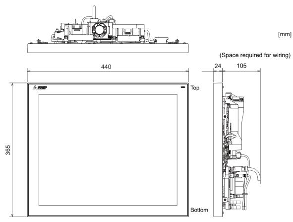
(Note) The figure above shows the state with the personal computer unit and the operation panel I/O unit mounted.
