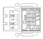
1pin Blue wire (cover notation: DA B) 2pin White wire (cover notation: DB W) 3pin Yellow wire (cover notation: DG Y)
