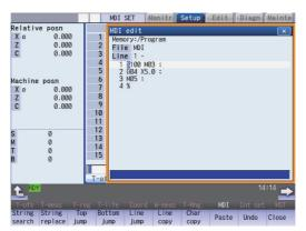
Program example (to rotate the spindle at 100r/min for 5 seconds)
