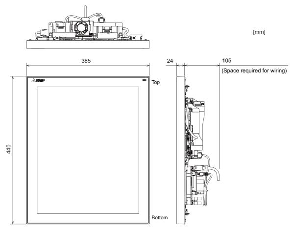
(Note) The figure above shows the state with the personal computer unit and the operation panel I/O unit mounted.
