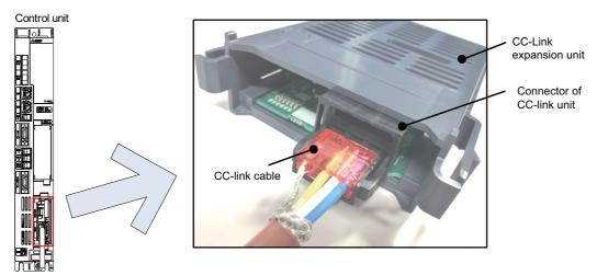
(Note) Connector of CC-Link unit is two-step structure. It is not different even if attach the cable to whichever.
