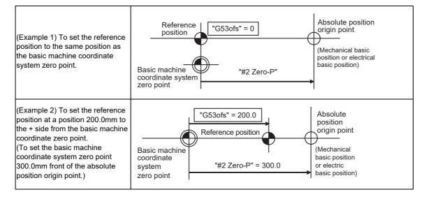
(3) When an MPI scale made by Mitsubishi Heavy Industries Machine Tool Co., Ltd. is used, set the zero point return parameters so that Z phase of the MPI scale becomes the grid point (electric basic position), and then perform zero point initialization setting.
