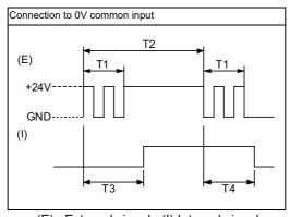
(E): External signal, (I):Internal signal
