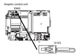
(Note) When installing emergency stop switch at operation panel and electric cabinet each, both emergency stop input signals (EMG), the signal at the graphic control unit side and at the control unit side, can be used.
