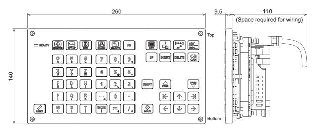
(Note) The above side view shows the state with the operation panel I/O unit mounted.
