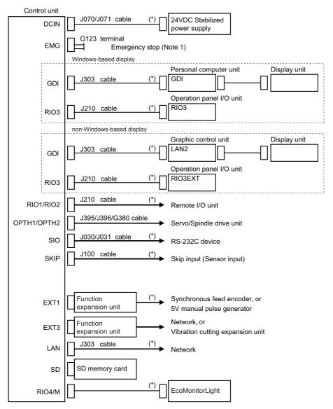
(Note 1) Use when installing an emergency stop switch in the electric cabinet. (Connection cable: J120 cable) When not used, connect the terminal connector (G123 cable).
