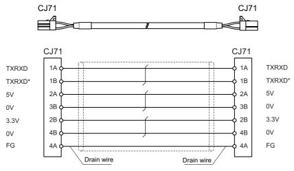
AWG22×3P (With shield / drain wire)
