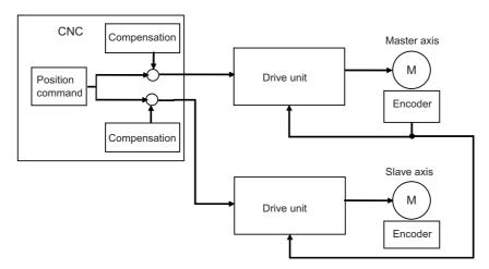
The "compensation" in the (1), (2) and (3) diagrams indicates the pitch error compensation, the thermal expansion compensation, the backlash compensation and the external machine coordinate compensation.
