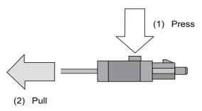
(f) For the Ethernet connector, pull off while holding down the locked latch.
