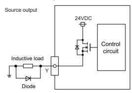
(Note 2) When the rush current exceeds the maximum output current, always connect a protective resistor (R=150 $\Omega$ ) serially to the load to suppress rush currents. Make sure that the current is less than the maximum output current including the momentary current.
