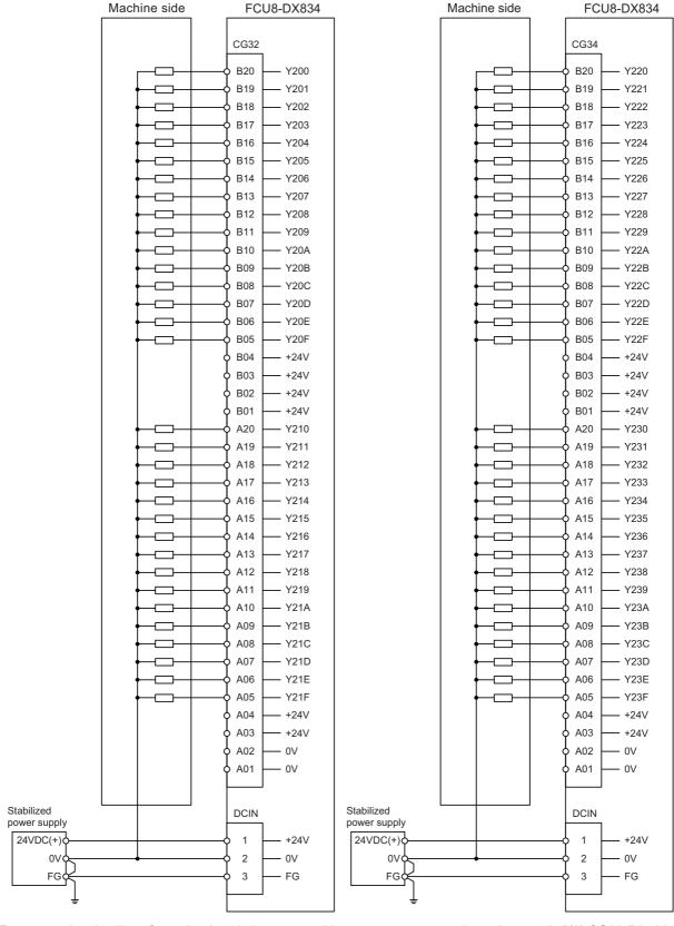
For connection details, refer to the descriptions on machine output connector pin assignment in "(2) CG32 (Machine signal output)" or "(4) CG34 (Machine signal output)" of "General Specifications: Operation Panel I/O Unit".
