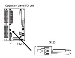
(Note) When installing emergency stop switch at operation panel and electric cabinet each, both emergency stop input signals (EMG), the signal at the operating panel I/O unit side and at the control unit side, can be used.
