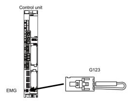
ISO13849-1 (PLd, Cat.3) and IEC62061 (SIL CL2) can be realized by using the safety remote I/O unit (directly wiring the external emergency stop redundantly).
