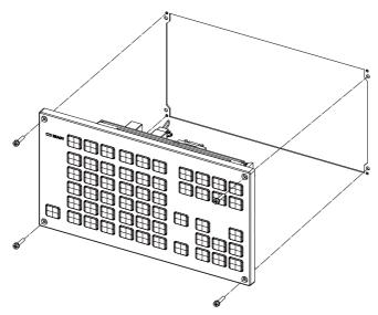
Fixing screw: Cheese head screw M3 (4 pcs). (Fixing screws are provided with the unit.)
