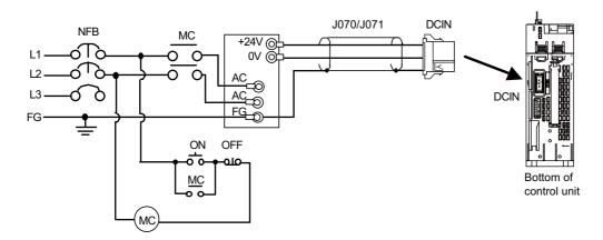
(Note 1) Rush current may occur to lead welding on the contacts, when a magnetic switch such as relay directly controls 24VDC's ON/OFF during 24V power supply to the control unit. Use relay with large heat capacity of contacts to control 24VDC's ON/OFF.
