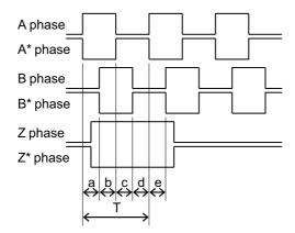
a.b.c.d.e: A phase or B phase rising edge (falling edge) phase difference = T/4 ± T/10
