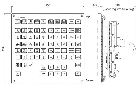
(Note) The above side view shows the state with the operation panel I/O unit mounted.
