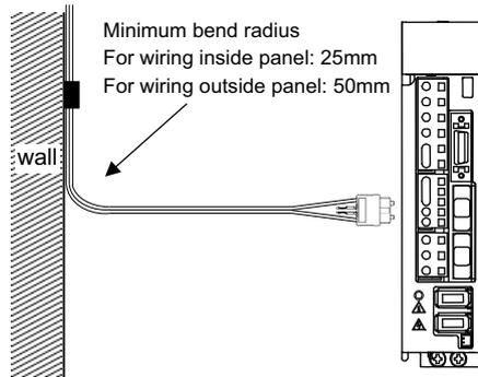
When laying cable, fix and hold it in position with using cushioning such as sponge or rubber which does not contain plasticizing material.
