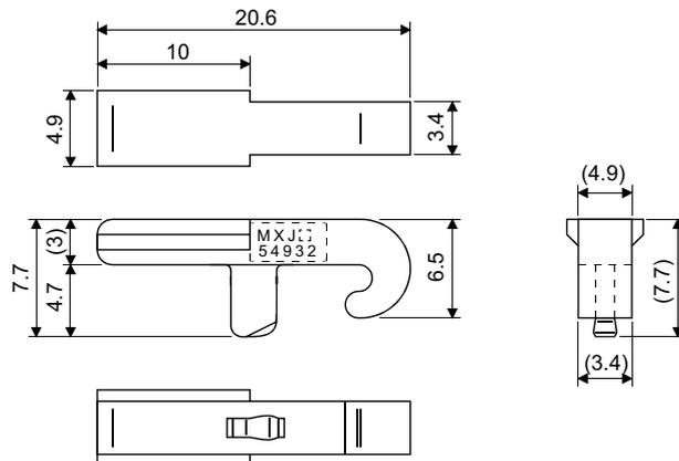
Appendix 1-3-2 Connector for servo and tool spindle
