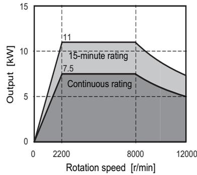
(Note) Actual acceleration/deceleration output is 1.2-fold of "Standard output during acceleration/deceleration" or 1.2-fold of "Short time rated output".
