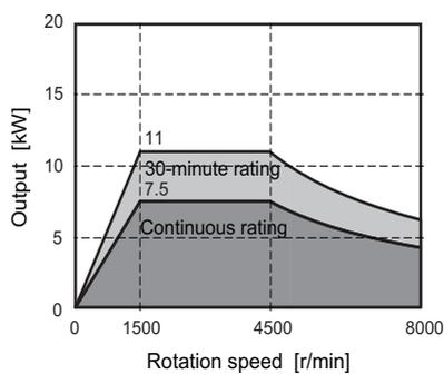
(Note) Actual acceleration/deceleration output is 1.2-fold of "Standard output during acceleration/deceleration" or 1.2-fold of "Short time rated output".
