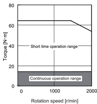
(Note) The above graphs show the data when applied the input voltage of 200VAC. When the input voltage is 200VAC or less, the short time operation range is limited.
