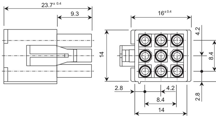
Spindle side encoder connector (for OSE-1024)
