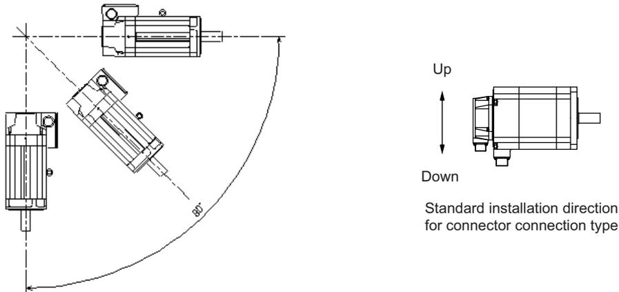
The spindle motor whose motor power line and detection lead wires are connected with connectors, as a standard, should be installed with the connectors facing down. Installation in the standard direction is effective against dripping. Measure to prevent oil and water must be taken when not installing in the standard direction.
