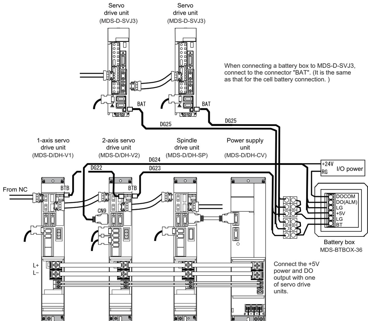
1. MDS-D-SVJ3 Series have no battery voltage drop warning signal input. Connect to CN9 of MDS-D/DH/DM Series servo drive unit.
