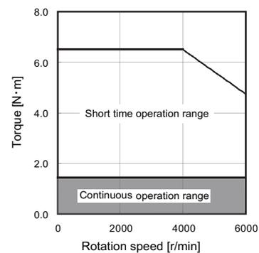
(Note) The above graphs show the data when applied the input voltage of 200VAC. When the input voltage is 200VAC or less, the short time operation range is limited.
