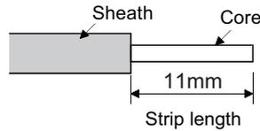
Retwist and straighten the core as shown below.
