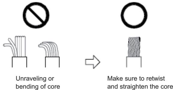
**(e) Wiring of the battery voltage drop warning output**
