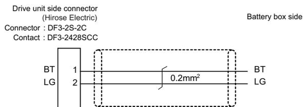
**CAUTION !** When DG24 cable is used, proximity switch or external emergency stop cannot be wired, so these functions cannot be used.
