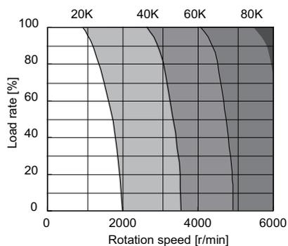
(Note1) The contour lines 20K to 100K in the graph indicate the temperature rising values from the start-up to saturation.
