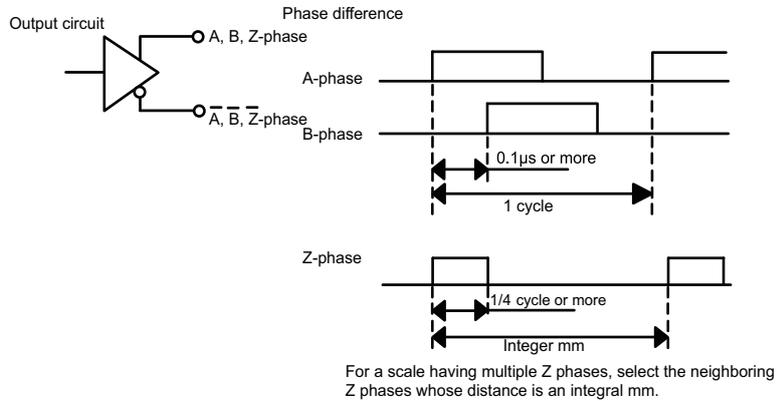
(Note)The above value is minimum value that can be received normally in the servo drive unit side.
