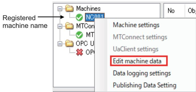
The editable screen differs depending on the selected machine type (NC type of "Machines", "MTConnect" or "OPC UA" in the tree of machines). The tab background of the uneditable screen is displayed in gray and those tabs cannot be switched. (In the screen below, "MTConnect Tag" and "OPC UA Tag" are not available.)
